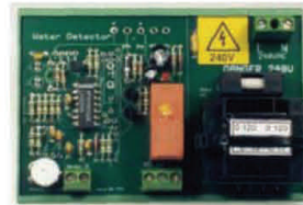
AT-LDM & AT-LDM-S open chassis, DIN rail mounting
