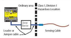
If protected by an agency approved zener barrier, TraceTek sensors in Class I, Division 1, Groups A, B, C, D Hazardous Locations (Zones 0 and 1 in Europe). Contact Tyco Thermal Controls to select proper zener barrier.
